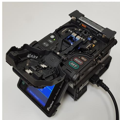
(b) Fibre splicer - used for joining fibres, our device is a Fujikura FSM-18S
