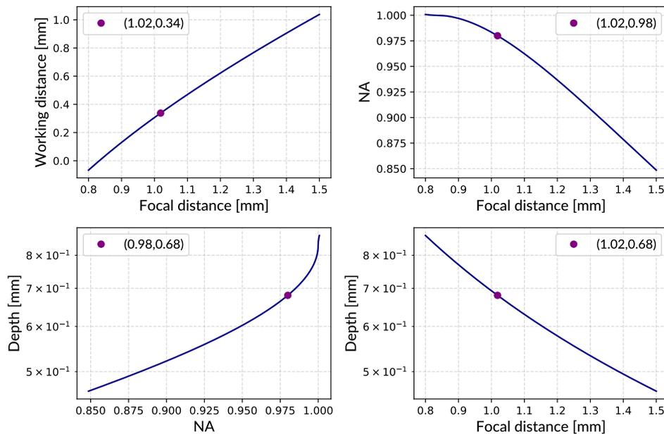
**Fig. 4.18.** The relation between the defining parameters of the parabolic mirror. Markers indicate the chosen values used in the mirror manufacture, with the coordinates given in the legend. These plots were generated by calculating the various parameters of the paraboloid as a function of a sensible range of input values of the other parameters, with a fixed mirror radius determined by the trapping beam diameter.
