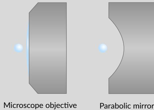
**Fig. 1.5.** Surface distance comparison between a microscope objective and a parabolic mirror trap
