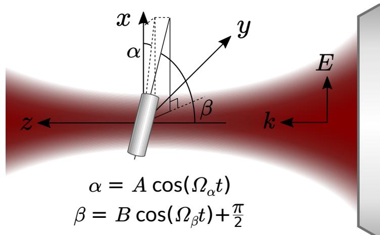
**Fig. 1.10.** A nanorod in a single beam optical trap. There are 5 degrees of freedom:  $x$ ,  $y$ ,  $z$  and  $\alpha$ ,  $\beta$ . The nanorod axis will oscillate harmonically about the polarisation axis  $\hat{E}$  in addition to the 3 translational oscillation frequencies.
