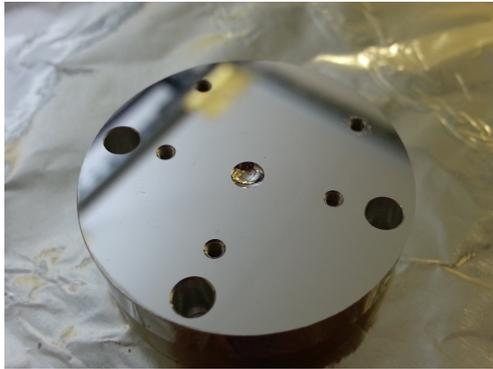
(a) Ellipsoidal objective mirror
