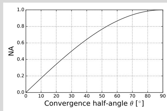
**Fig. 1.6.** NA as a function of convergence angle
