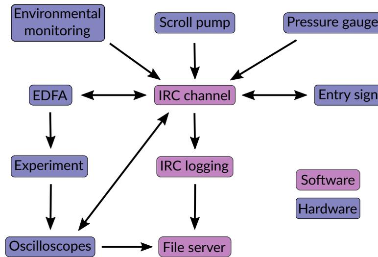
**Fig. 4.27.** Systems level overview of the lab - Information flow and centralised logging architecture for the various hardware in the lab
