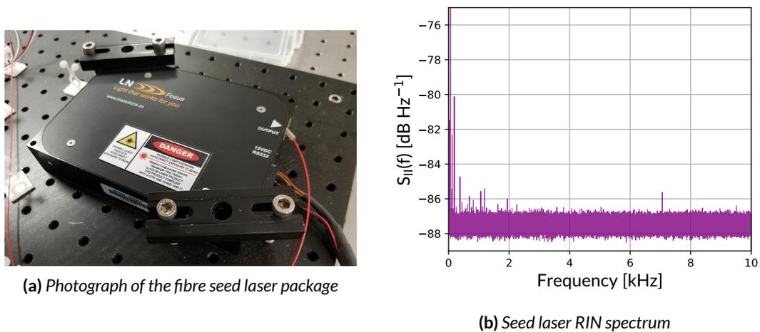
Fig. 4.6. Seed Laser photo and RIN specification
