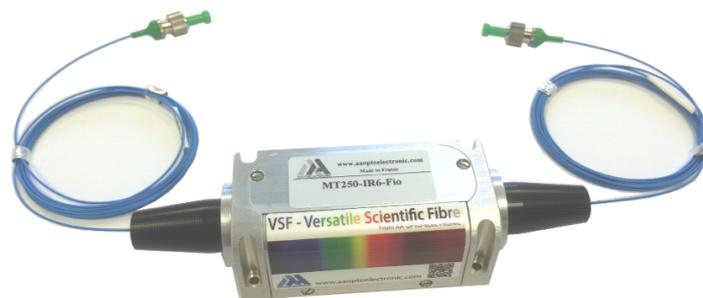
**Fig. 4.11.** The AOM package - This is a single mode fibre coupled device that transmits the first diffracted order with a power related to the RF driving power. This device acted as an intensity modulator and frequency shifter for use when performing heterodyne measurement.
