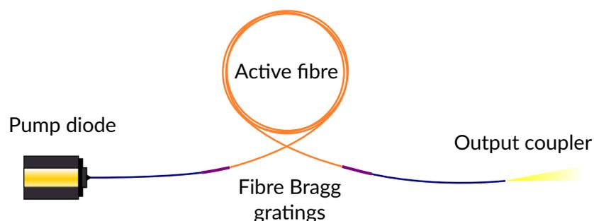
Fig. 2.18. The main components of a fibre laser
