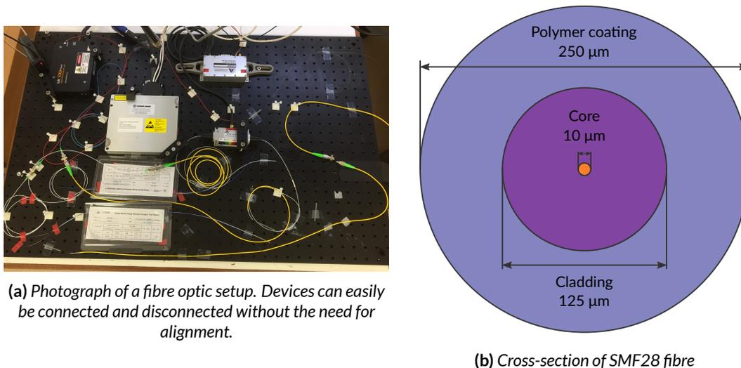
**Fig. 4.3.** Setup illustration and cross-sectional diagram of the fibre optics used in this project.
