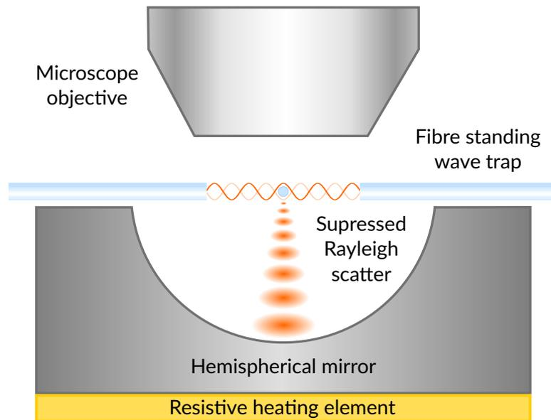
**Fig. 7.3.** Rayleigh scatter suppression geometry - A standing wave trap confines the particle in three dimensions at the centre of a hemispherical mirror. Rayleigh scatter is suppressed by the correctly sized mirror, reducing RPSN.
