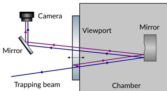
**Fig. 4.25.** Generation of the etalon pattern used for detecting changes in pressure at close to atmospheric pressure. Light reflected inside the viewport glass interferes with that which passes straight through to give an interference pattern that depends on the position of the glass-air interface. Angles have been exaggerated for clarity.
