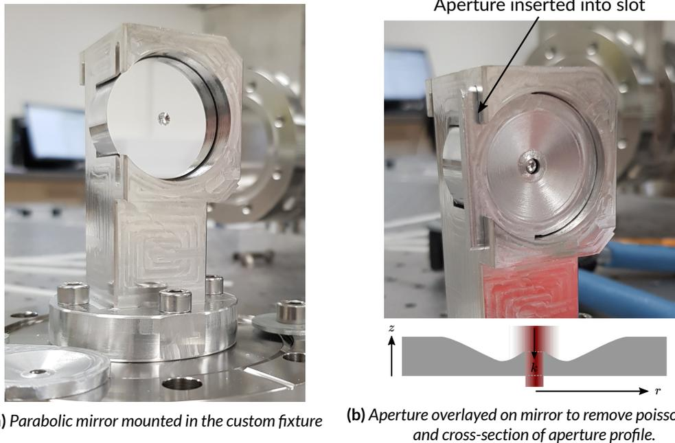
**Fig. 4.19.** Parabolic mirror objective - The optic is shown in its custom mount with and without the custom aperture used to block the Poisson's spot.
