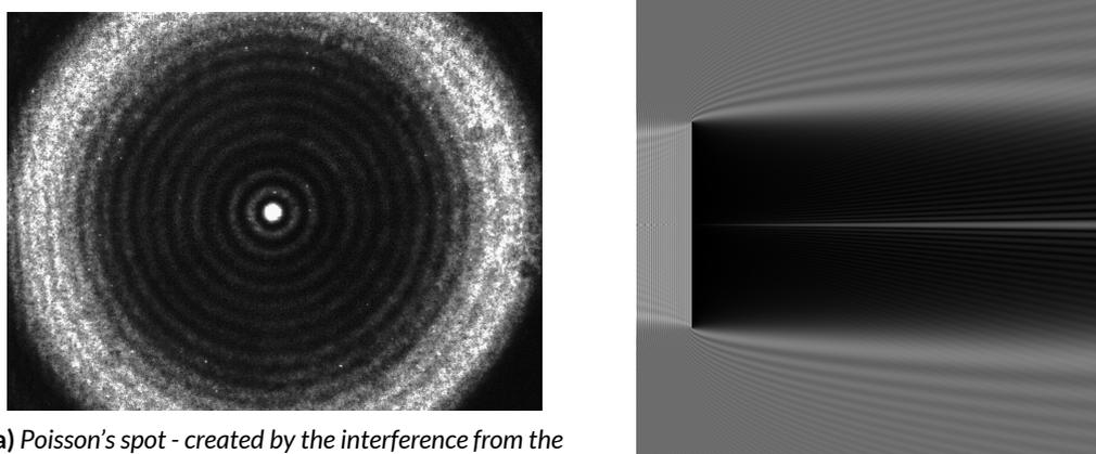
**Fig. 4.20.** Poisson's / Arago's / Fresnel's spot - An optical artifact created by the diffraction of the laser at the edge of the parabolic mirror section. An unexpected central bright spot is produced.
