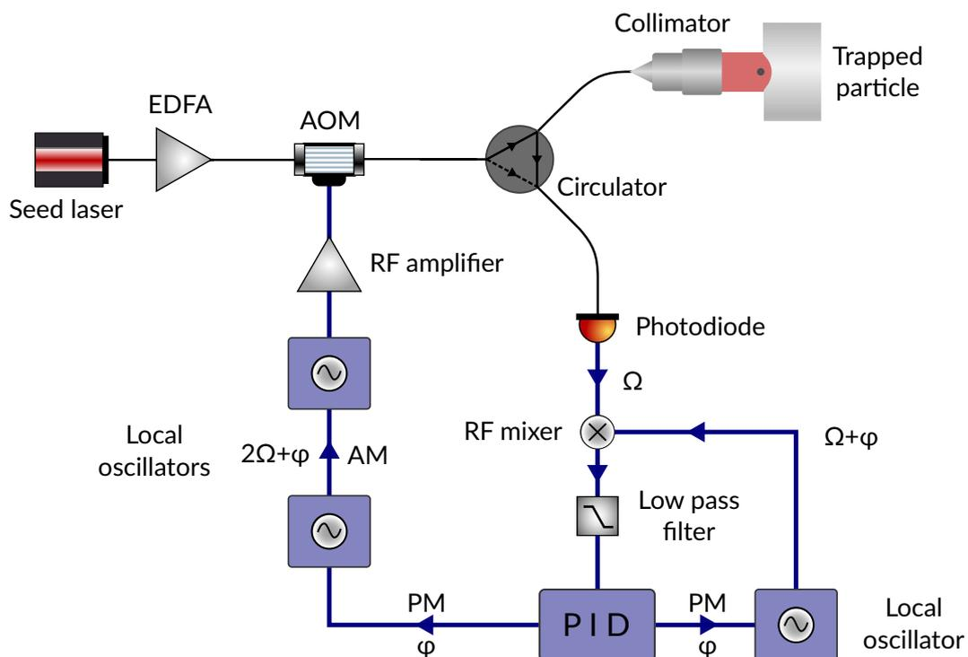
Fig. 7.1. PID cooling system schematic
