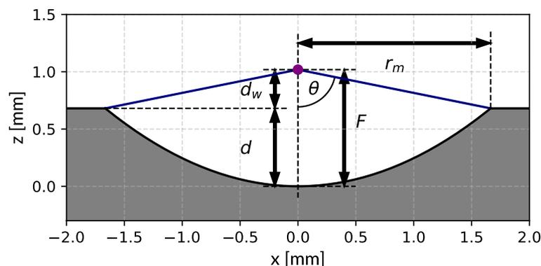
**Fig. 4.17.** Specification of the parabolic mirror - The parabolic mirror is defined by the mirror section radius  $r_m$ , focal length  $F$ , depth  $d$ , working distance  $d_w$  and NA which is related to angle  $\theta$ .
