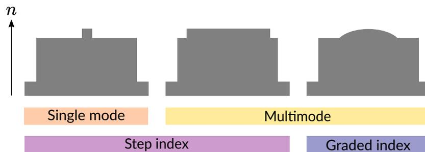
Fig. 2.15. Optical fibre refractive index cross-sections
