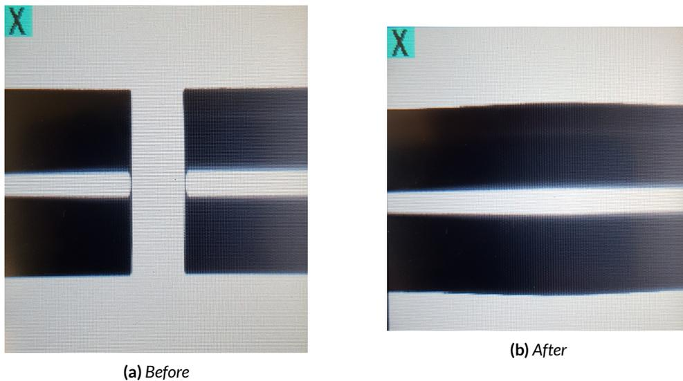
**Fig. 4.5.** Fibre fusion splicing - fibre is joined under a microscope so that it forms a continuous piece of glass. The splice point is visible only as a small region of slightly increased radius and losses were not measurable with the available photodetectors.
