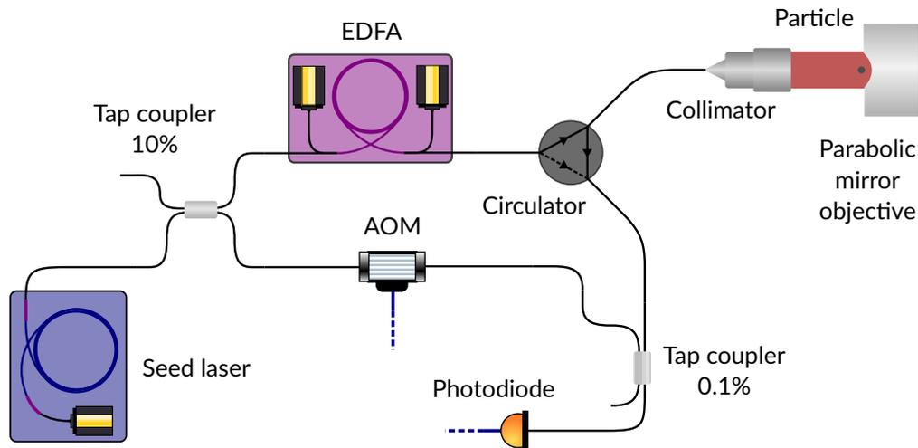
Fig. 4.2. The optics subsystem setup for heterodyne measurement
